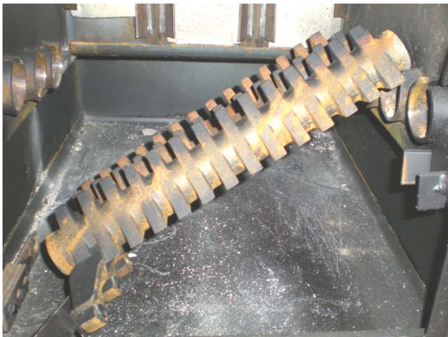
Figure 1.5.5. The grate elements are dismantled from their supporting foot-steps;
