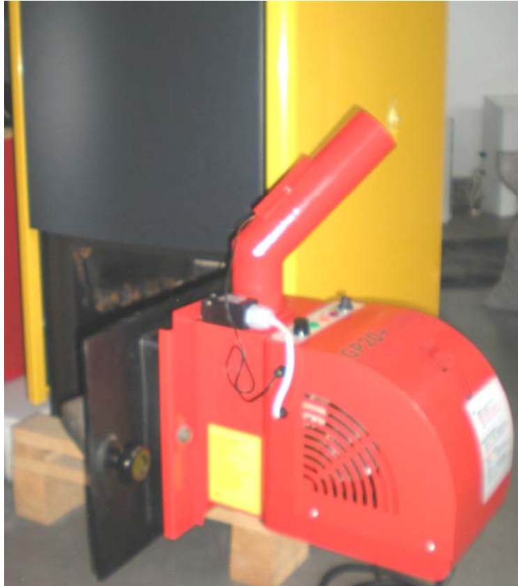
Figure 1.5.7. The automatic pellet burner “ERATO GP20+” is mounted on the specially designed front door of the boiler;
