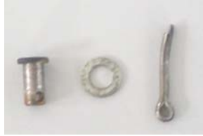
Figure 1.5.4. Fixing splint pit, washer and axis, detached from the grate moving mechanism of the boiler;
